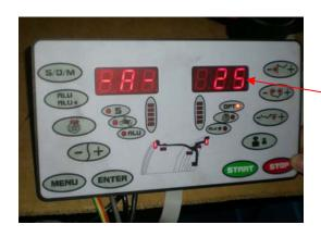
In the mode of the diagnosis of distance "A" potentiometer, adjust the potentiometer to 25 which is shown in the screen. Please note the gauge should be in the "zero" position
