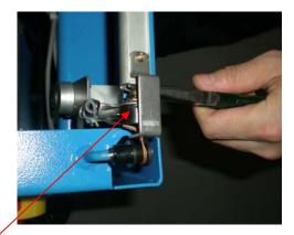
In the mode of the diagnosis of the distance "D" potentiometer, adjust the potentiometer to 25 which is shown on the screen. Please note the gauge should be in the "zero" position.
