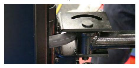
Insert the Bead Roller Arm (Part 1) into the Bracket and replace the support pin and locking nut as shown.
