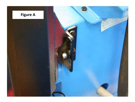
Use the Rear Column attachment and bolt (Part 5) to attach the column mounting plate onto the Rear Mounting Extension Bracket (Part 7) as shown. (Figure A)
