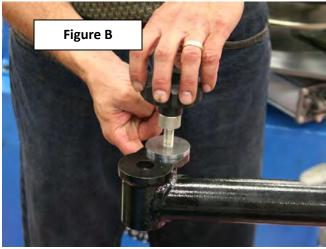
Remove the Bead Roller Arm support pin (Figure A) and Locking Nut (Figure B) from the support bracket
