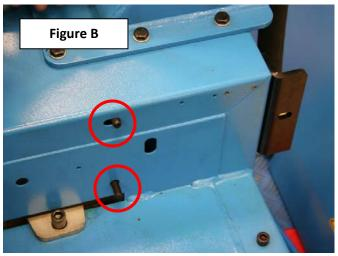
(Figure A) Locate the Front Column Attachment and Bolts (Part 6) and insert the bolts through the holes from the inside of the tire changer as shown. (Figure B)
