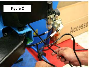
Locate the 6mm Air Hose at the base of the RHA-SA and feed it to the inside of the tire changer from the backside inlet. (Figure C)
