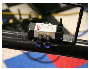
Remove the control Switch cover plate to reveal the Air Line auto-lock unions and attach the 3 colored air hoses to the auto-locking hose fittings on the control switch as shown below. (Figure A)
