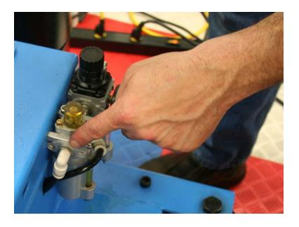
Locate the air line that is connected to the oiler, and follow this line to the inside of the tire changer.
