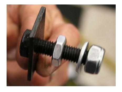
Locate the Rear Column attachment and bolt. (Part 5)
