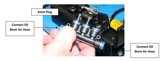
Connect each end of the **8mm** air line; **previously cut**, into the 5-way auto lock union valve **(Part 4). Note:** If you are not using more than one pneumatic accessory, an extra **6mm** plug will be provided.
