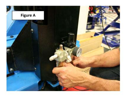
Attach the Oil/Air Regulator onto the side of the RHA-SA via the predrilled holes, (Figure A) and re-attach the previously marked air lines to their respective attachments. (Figure B)
