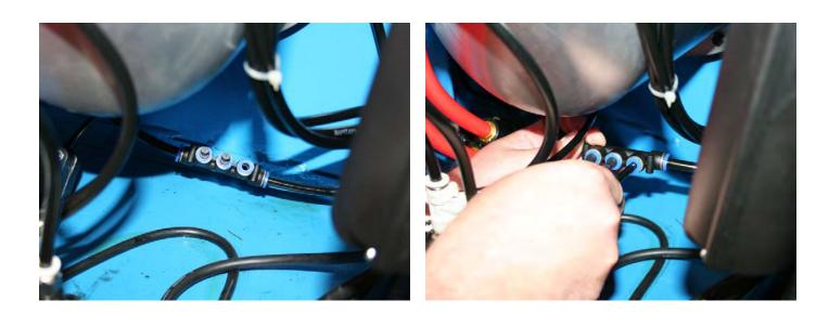
Insert 6mm air line into the 5-way auto lock union valve (Part 6) and use the provided 6mm plugs to plug up the unused spaces in the 5-way auto lock union valve (Part 6).
