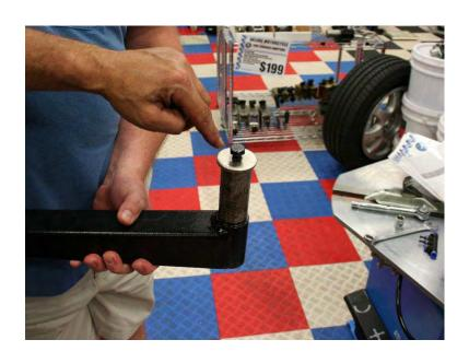
Locate the Bead Lifting Disc Arm (Part 3) and fit the arm into the bracket. (Figure A)
