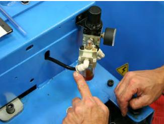
Remove the attached Air hoses from the Oil/Air Regulator that will be located on the side of your tire changer.
