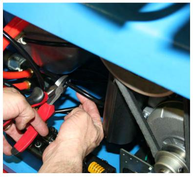
Once you follow the air line from the oiler to the inside of the tire changer cut this air line.
