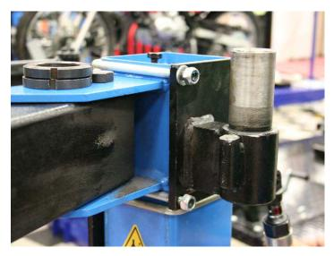
Bolt the Support Arm Bracket (Part 5) onto your Tire Changer's Vertical Support Column using the U Bolt set (Part 2).
