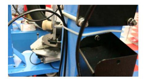
Take the longest **6mm** air line and route it to the back of the column. Secure the air line to the column **(Ties not included).** Route the airline to the back of the tire changer and insert it into an opening.
