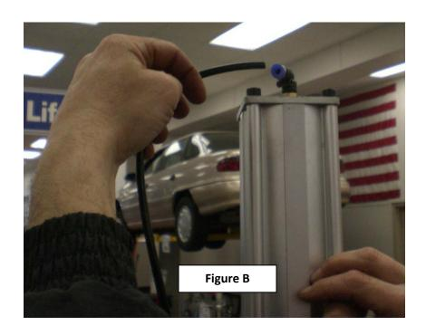
Insert the second longest hose into the **6mm** auto lock union located on the top of the cylinder **(Part 1)**.
