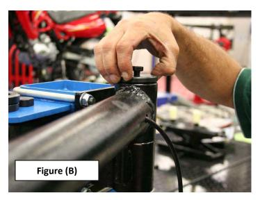
Place the 2 part curved support arm (Part 4) onto the support arm bracket (Part 5). Secure the Arm with the provided washer and bolt. See (Figures A & B)
