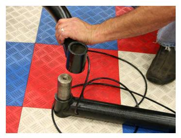
For packaging, the ERHA-BP is configured in the reverse position. In order to properly mount the 2 Part Curved Support Arm (Part 4) onto the right side of the tire changer the arm must be reversed on the center hinge bracket as shown. Remove the bolt and washer, flip the curved section of the arm over, and remount the section onto the hinge bracket in order to properly configure the arm.
