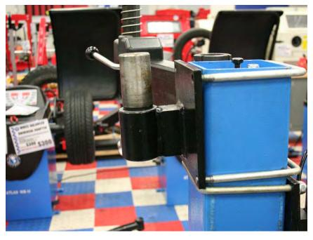
The ERHA-SA is furnished with a U-Bolt set (Part 2). Use the U-Bolts to attach the ERHA onto the Vertical Support column of your Tire Changer. See (Figure A)
