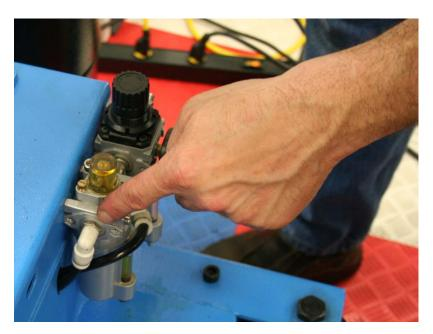
Locate the air line that is connected to the oiler. Remove the access panel on your tire machine and follow this line to the inside of the tire changer.
