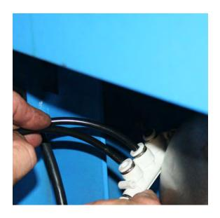
Insert 6mm air line into the 5-way auto lock union valve (Part 6) and use the provided 6mm plugs to plug up the unused spaces in the 5-way auto lock union valve (Part 6).
