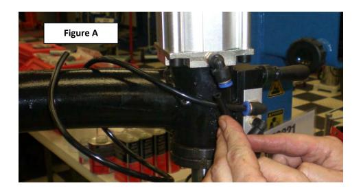
There are three **6mm** air lines attached to the air valve/curved support arm **(Part 4)**. Insert the shortest air line into the **6mm** auto lock union located at the base of the air cylinder. **(Figure A)**
